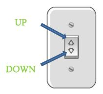
Motorized shutters come with several switch styles and remote options. We highly recommend a "momentary" style switch that requires you to actually hold the switch while the shutter opens and closes.
