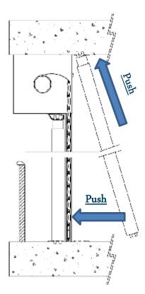
If storm bars (inner or outer) are installed on your unit, it is imperative that they be installed properly and in place during windy conditions, especially storm conditions.
